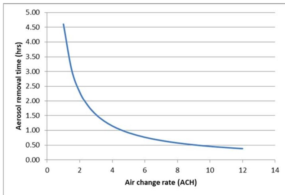
FIGURE 1: Relationship between time to remove 99% of aerosol with ventilation air change rate.
